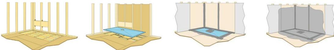
ARC TrueDek Classic Bases are structural, pre-sloped pans available in 15 different sizes with a 4" square drain. This product is 7/8" thick and
